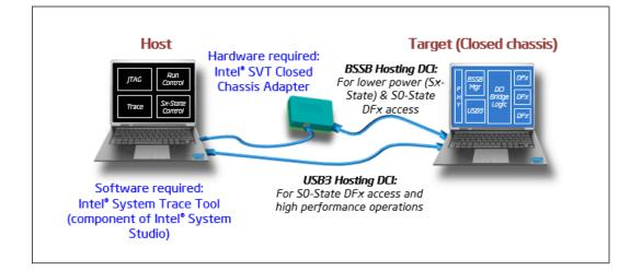
Figure 33-2. Platform Setup with DCI Connection
