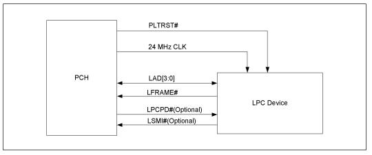
The PCH supports all of the signals that are shown as optional, but peripherals are not required to do so.
