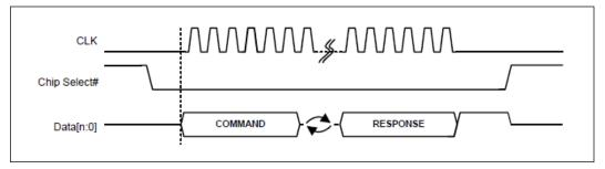
An eSPI transaction consists of a Command phase driven by the master, a turn-around phase (TAR), and a Response phase driven by the slave.
